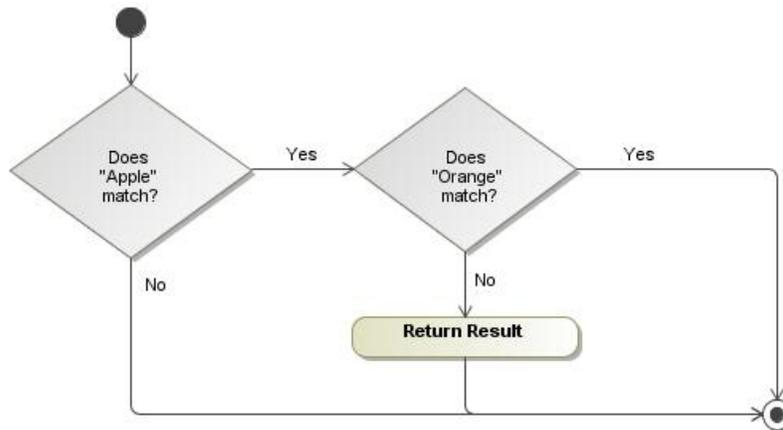
Figure 8: NOT Operator Logic
