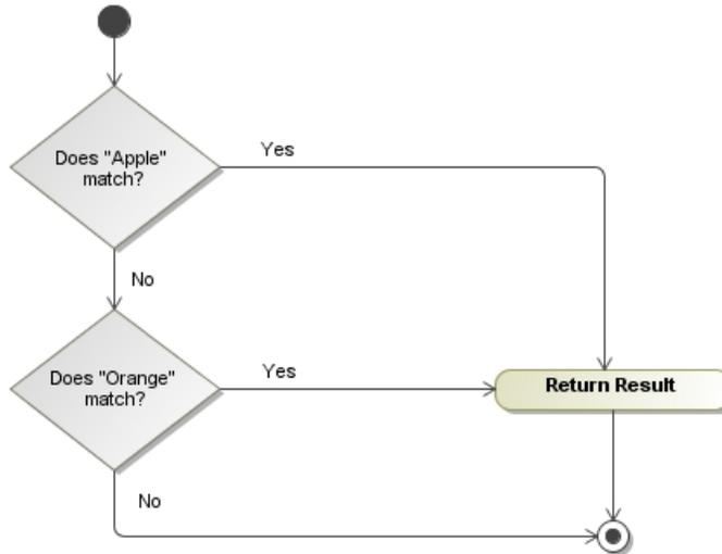
Figure 7: OR Operator Logic
