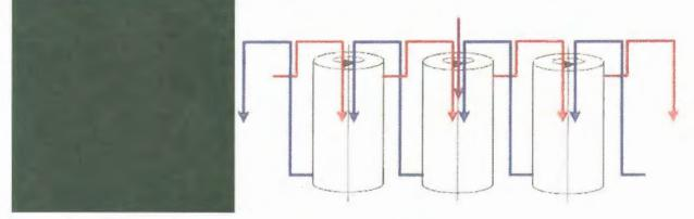
Since the cascade is exponential, its length is approximately a logarithm. Each stage is an appropriate number of centrifuges in parallel.
